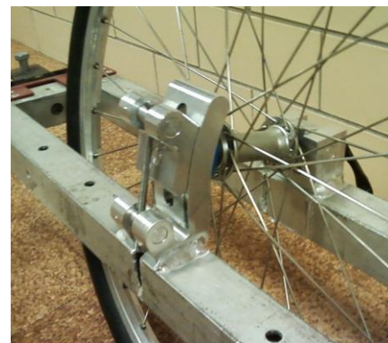
Figure 3: Cylindrical dropout to adjust the camber angle
