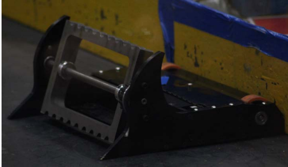
Figure 1 Horizontally spinning ‘blade’ attached to the front of the robot
