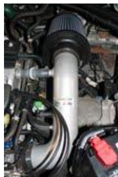
Figure 3: Intake after modification
