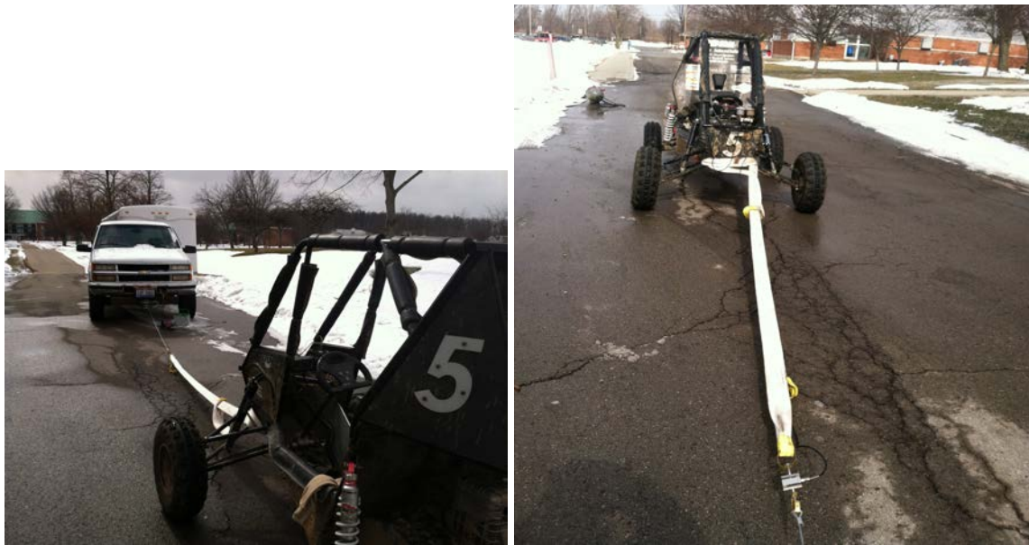
Figure 1: Test surface and set up. Load cell visible in right photo.
