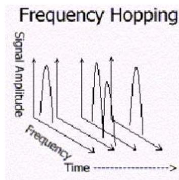
**Figure 5.** Spreading the spectrum in FH-CDMA
