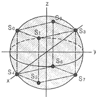
**Figure 1.** An example of a three dimensional constellation diagram for OFDM
