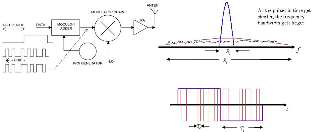
**Figure 4.** Spreading the spectrum in DS-CDMA
