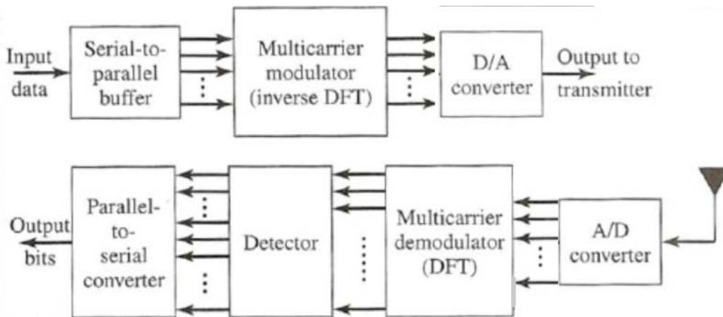
**Figure 2.** A simplified block diagram of an OFDM transmitter/receiver
