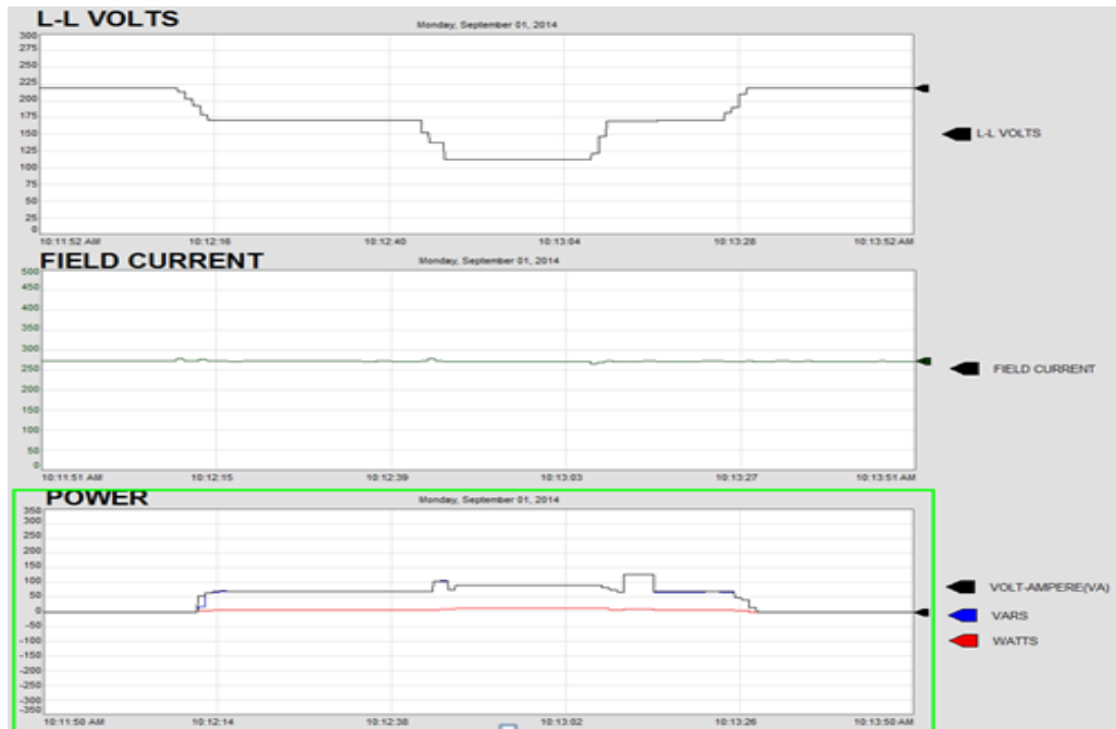
Figure 8: Lagging power factor load with the field current held constant (manual mode)
