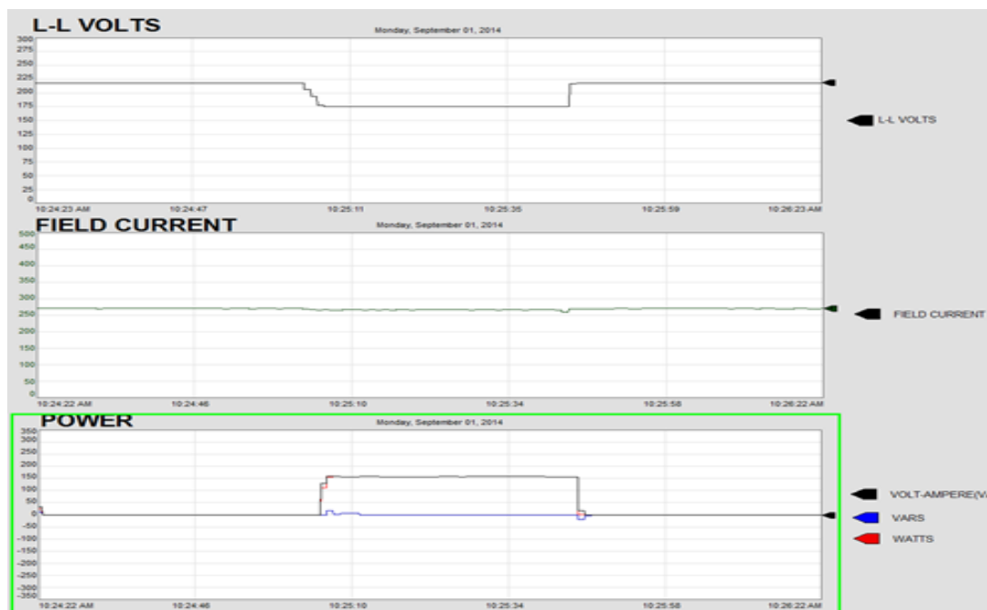
Figure 6: Unity power factor load with constant field current (manual mode)
