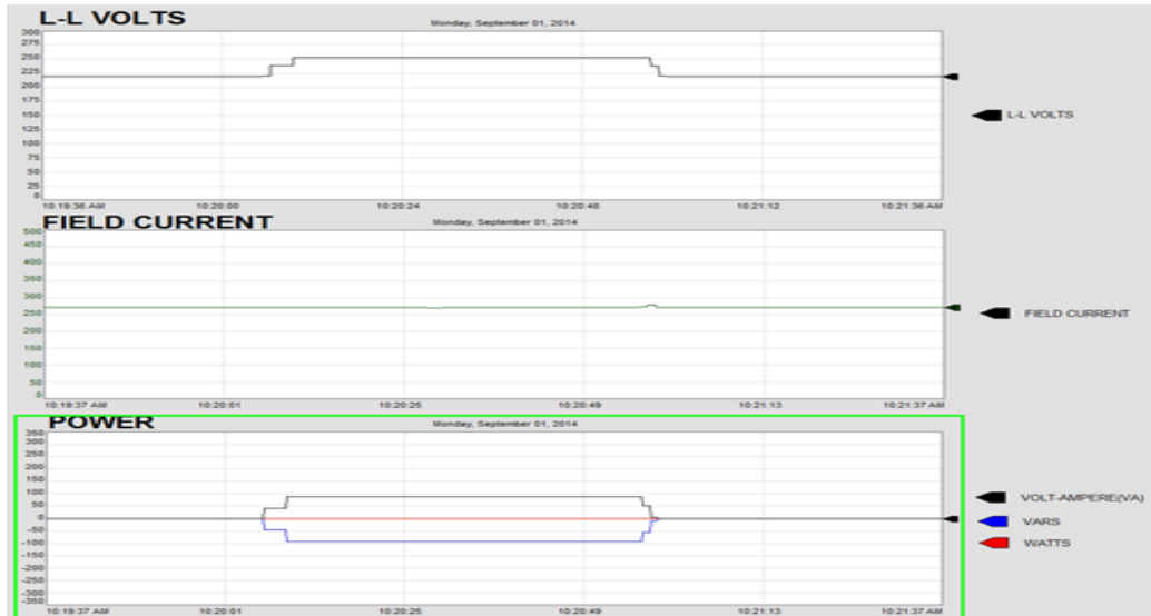
Figure 10: Leading power factor load with the field current held constant (manual mode)
