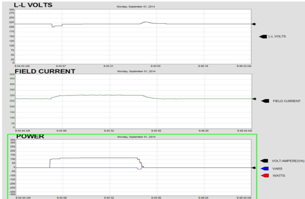
Figure 1: Unity power factor load with AVR (automatic mode)
