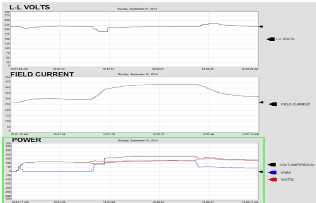
Figure 13: RLC load with AVR (automatic mode)
