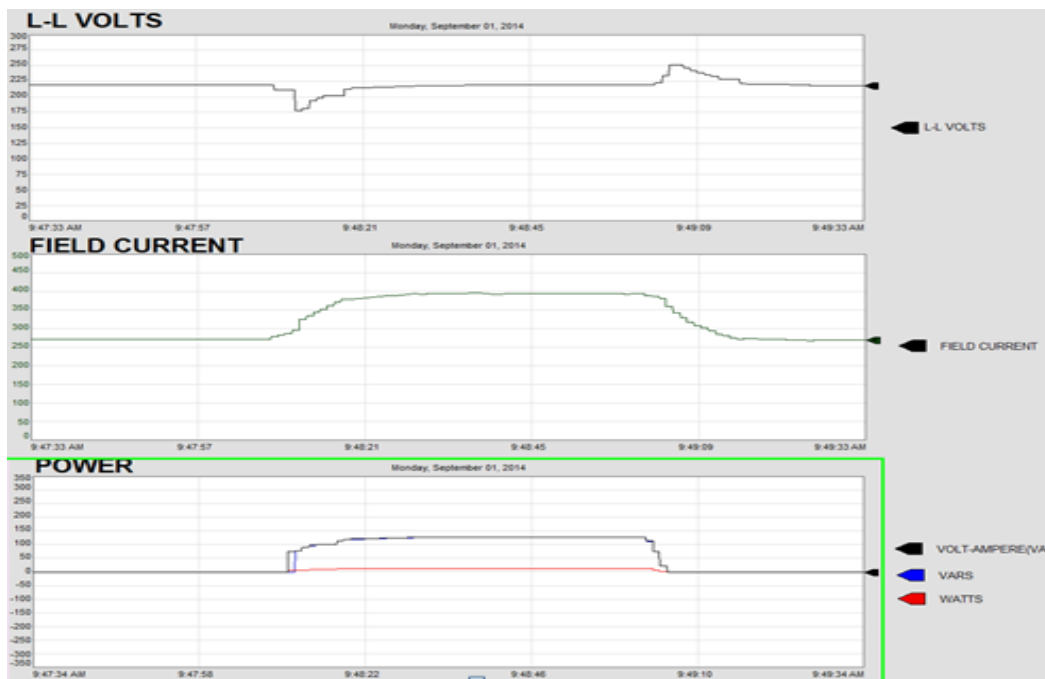
Figure 9: Lagging power factor load with AVR (automatic mode)
