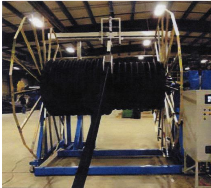
Figure 3: Assembly view of the winding coil machine, wheels, and spool [3]
