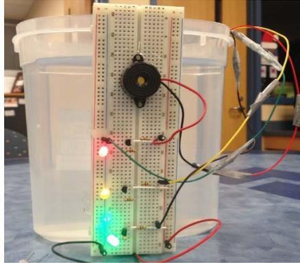
*Figure 3: Sensor developed to measure levels of water inside a tank. At level 3, which indicates the tank is full, the attached buzzer alarm goes off simultaneously as the red indicator light comes on*
