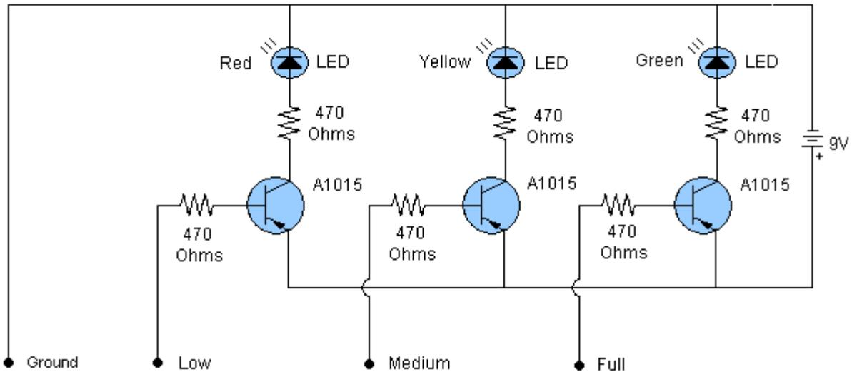
*Figure 2: Circuit diagram for water level indicator<sup>13</sup>*
