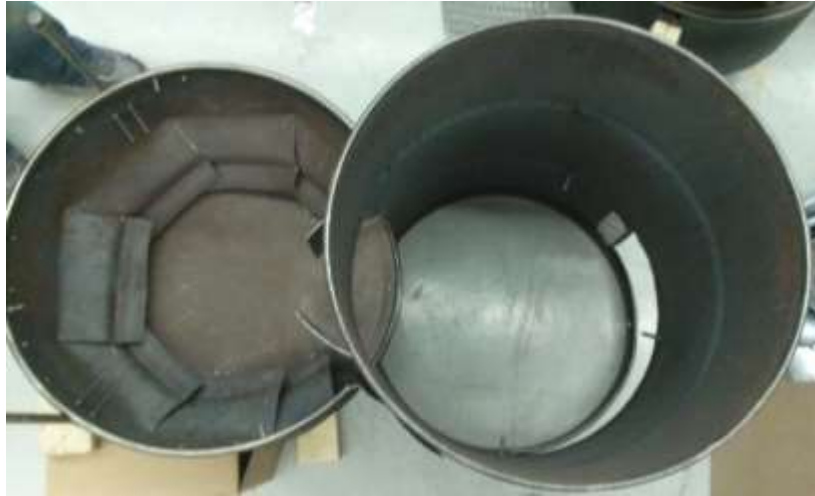
Figure 19: Smoking Chamber - Cooking Surface Mate (Before Bolting)
