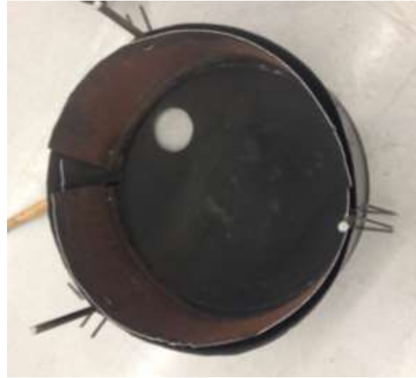
Figure 3: Cutting the second barrel with nibbler Figure 4: Simple stove with insulation
