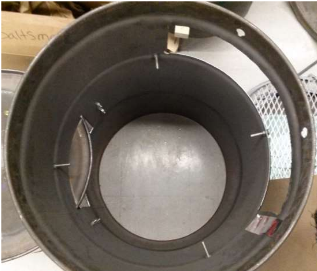
Figure 20: Smoke Chamber- Cooking Surface Mate (After Bolting)
