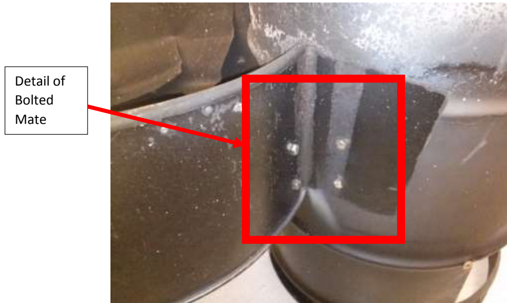
Figure 15: Bolted Mate Detail
