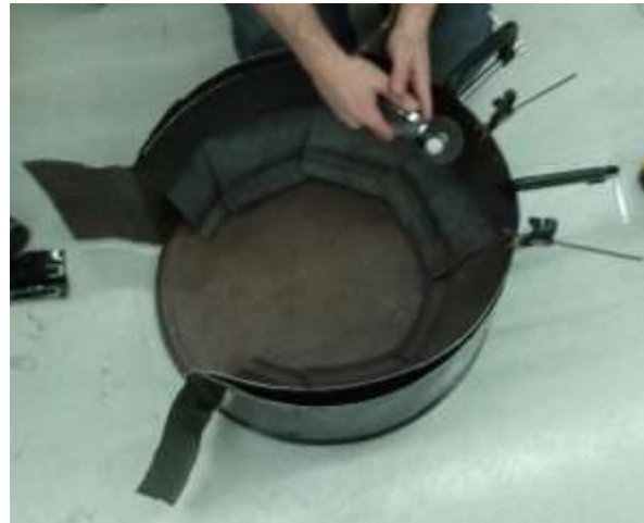
Figure 9: Installation of Heat Funnel
