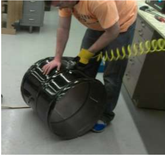
Figure 3: Cutting the second barrel with nibbler Figure 4: Simple stove with insulation
