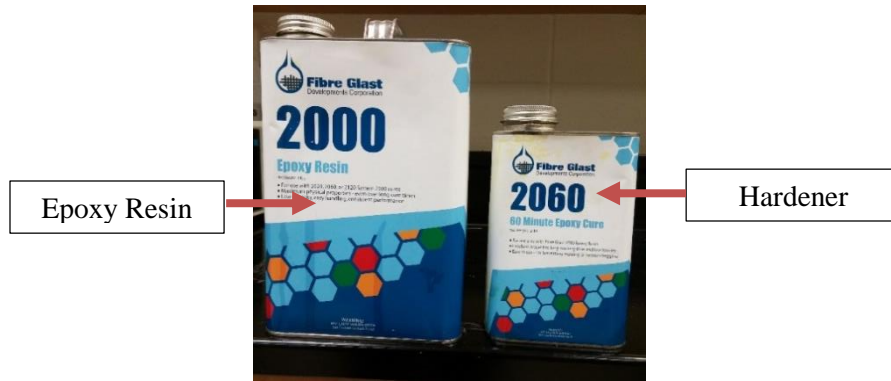
Figure 3 Fibre Glast Epoxy Resin and Hardener forms the matrix of the fiberglass composite
