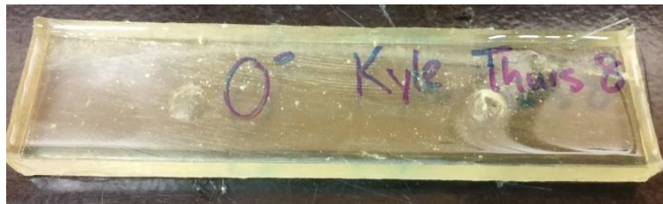
Figure 5 Reinforced fiberglass composite made by a student
