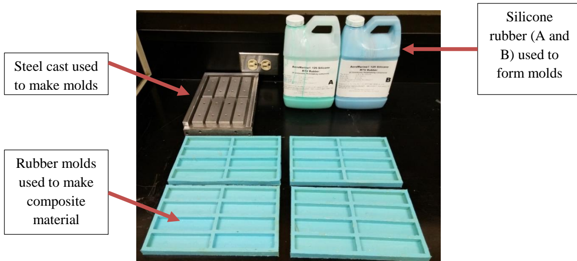
Figure 2 Silicone rubber molds for laying the composites
