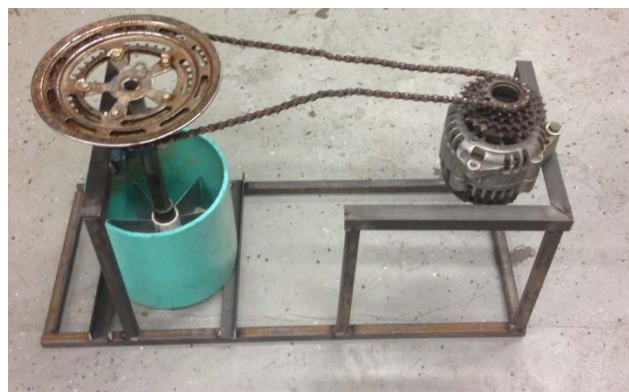
Figure 5. The assembled turbine and generator
