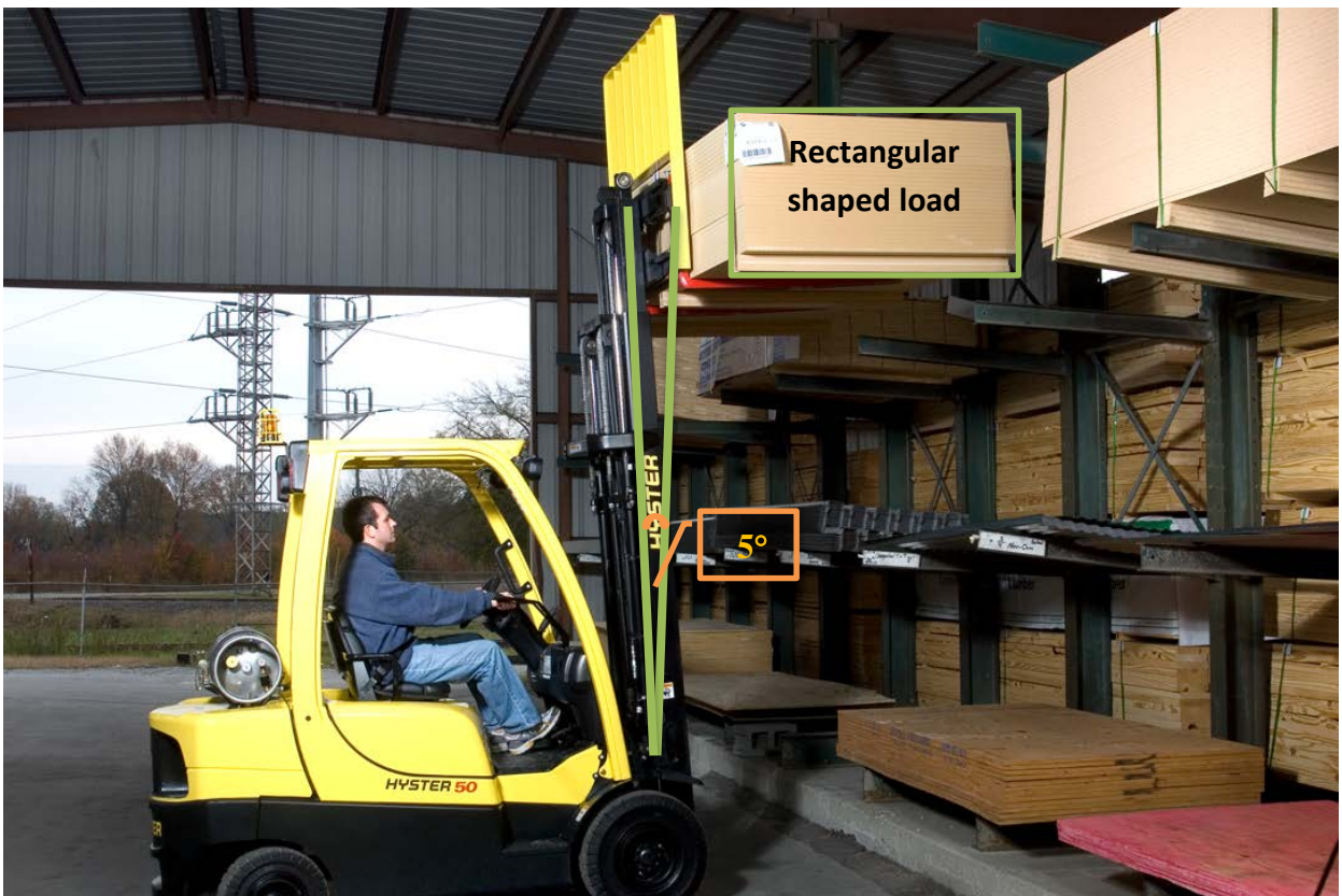
Figure 10 Hyster forklift in operation similar to Figure 5 Tilted 5^\circ back with large rectangular shaped load
