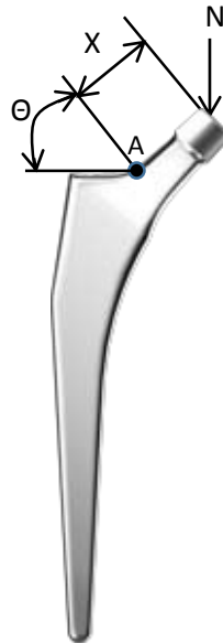
Figure 2: Simplified Free Body Diagram of Hip Implant
