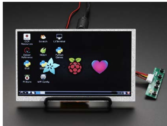
Figure 5: Vehicle Map Display - 7", 800x480 through HDMI connection
