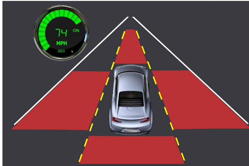
Figure 6: Vehicle map rendering showing that the system sensors detect an object on all sides of the car
