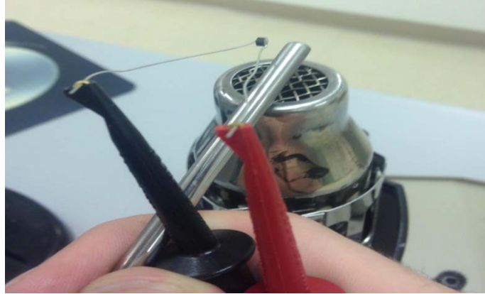
Figure 6: Testing Thermistor for the Overheating Car Alarm Circuit
