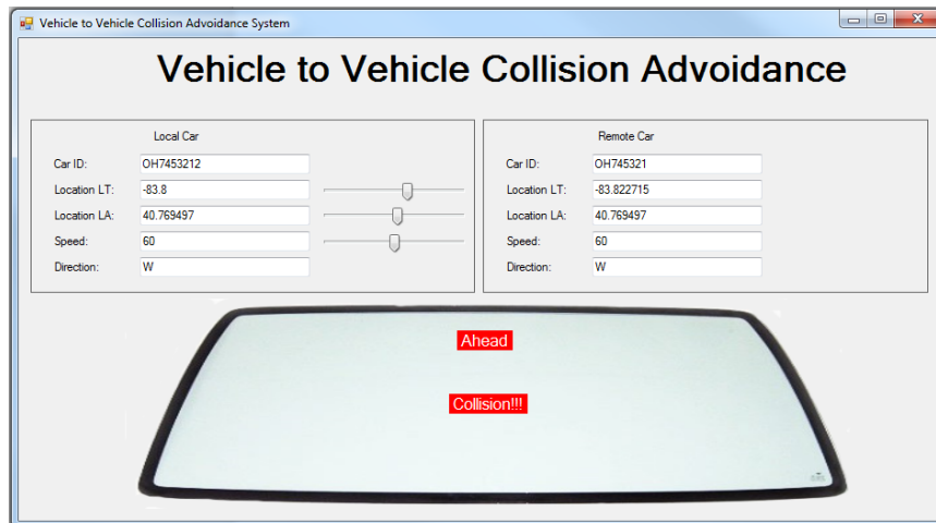
Figure 6: The user interface shows a heads up that a collision has occurred in the front of the vehicle.
