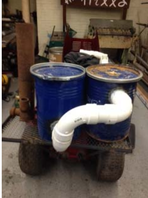
Figure 4: Filters and PVC Piping.
