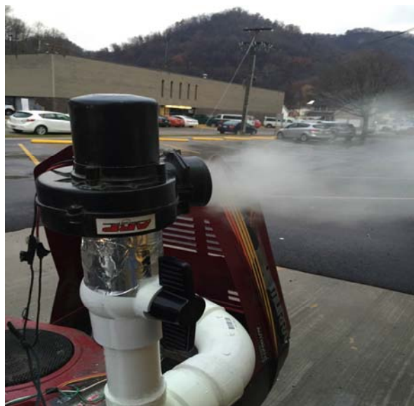
Figure 11: Syngas exiting the fan.
