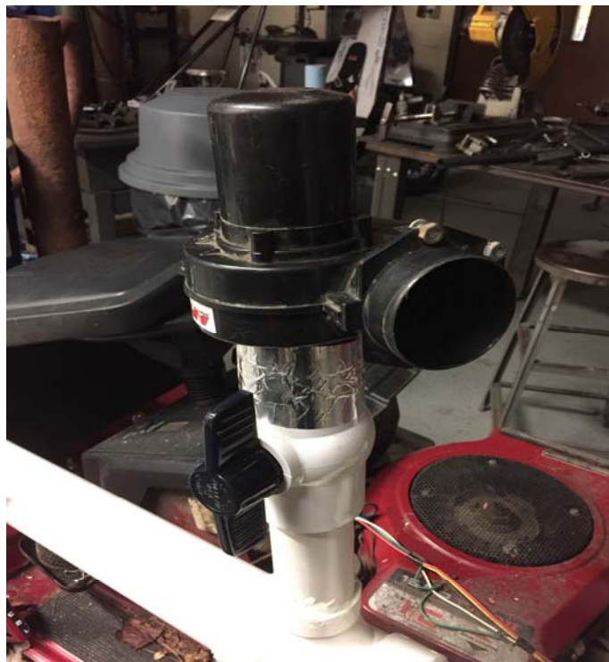
Figure 7: Ball valve and electric fan.
