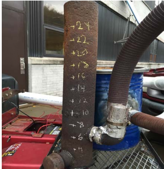
Figure 12: Fire tube with marks that are two inches apart.
