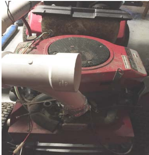
Figure 8: 90 degree PVC pipe routed into the carburetor.
