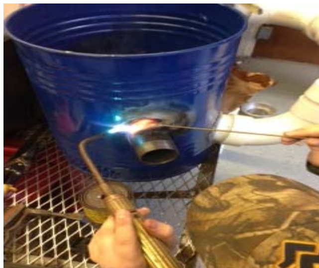
Figure 3: Brazing metal pipe to filter.
