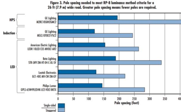
Figure 11. Pole Spacing [6]
