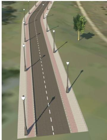
Figure 12. Staggered Positioning of Streetlights (Image from Elliot Rosenfield Autodesk Blog)
