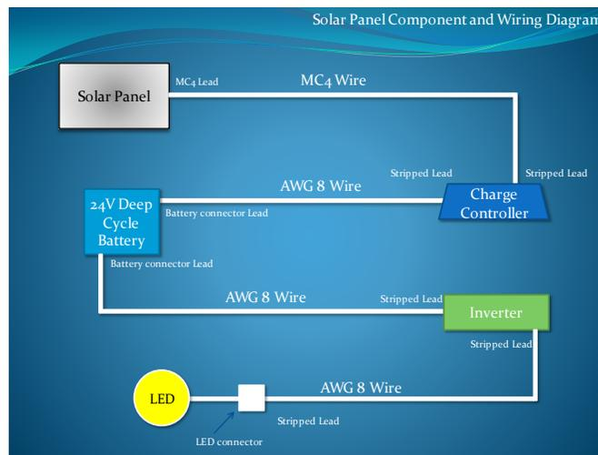
Figure 15: Solar Panel Component Wiring Diagram
