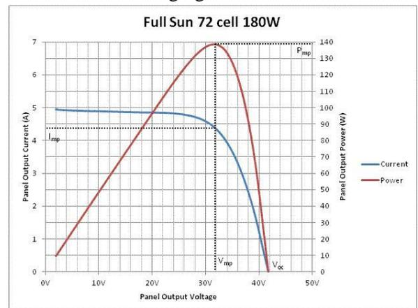
Figure 16 - Solar Panel Power Curve
