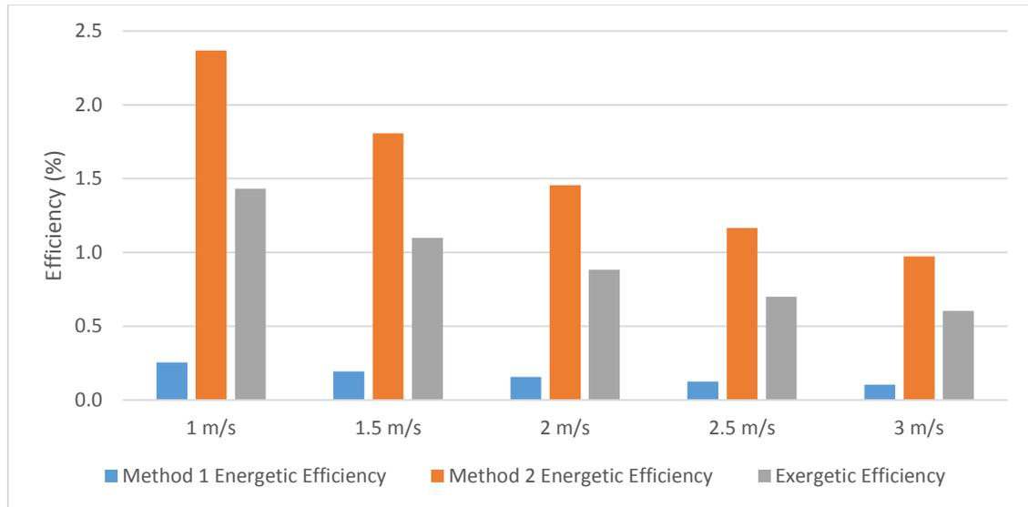
Figure 4: Energetic vs. Exergetic efficiencies for FC drying.
