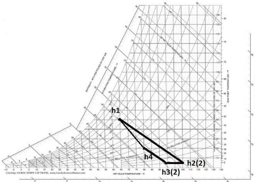
Figure 2: Psychrometric chart plotting the processes of method 2.
