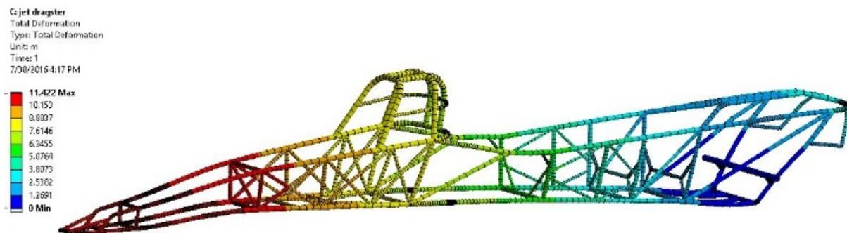
Figure 1: Static structural simulation of jet dragster impact
