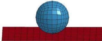
**Figure 2:** Ball impacting plate
