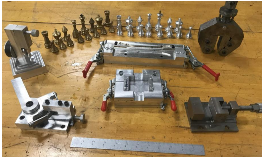
Figure 5. Air Engine, Chess Set, Toggle Clamp, Tensile Fixture, Vice, and Material Testing Sample Fixtures.
