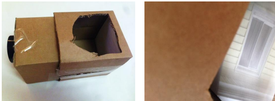
Figure 4: Camera obscura made using a disassembled camera lens (left) and an example of an image it can create (right).
