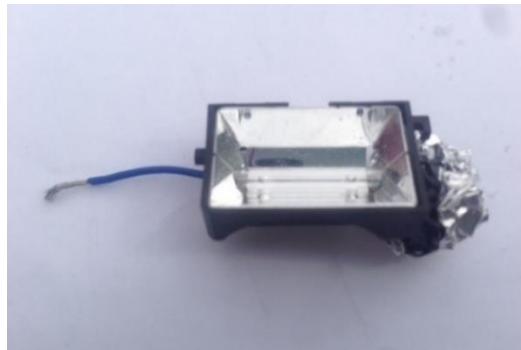
Figure 5: Static electricity detector using a flash tube.
