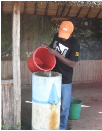
FIGURE 2: TYPICAL HOUSEHOLD SAND FILTER IN SAINTE LUCE, MADAGASCAR
