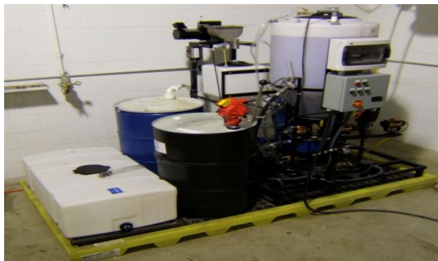
FIGURE 5 AUTOMATED BIODIESEL CONVERSION SYSTEM
