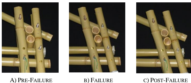
FIGURE 7 RIGHT COLUMN-ROOF JOINT EDGE BEARING FAILURE OF LOWER OUT-OF-PLANE MEMBER.
