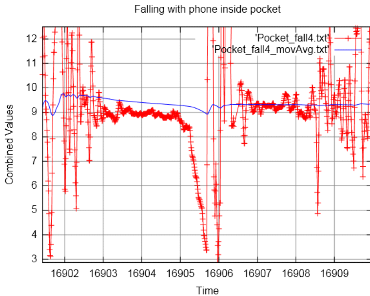
Figure 5: Data from a subject who stood still then proceeded to fall onto seat cushions
