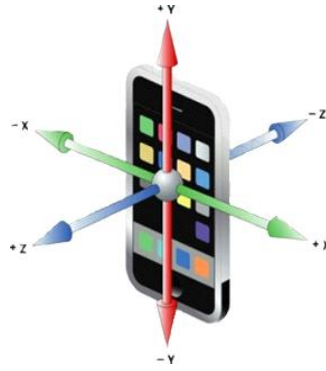
Figure 1: This shows the axes of the phone in respect with the accelerometer embedded onto the smart phone.
