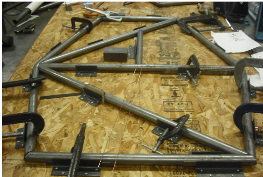
Figure 8: Vehicle firewall being built on jig
