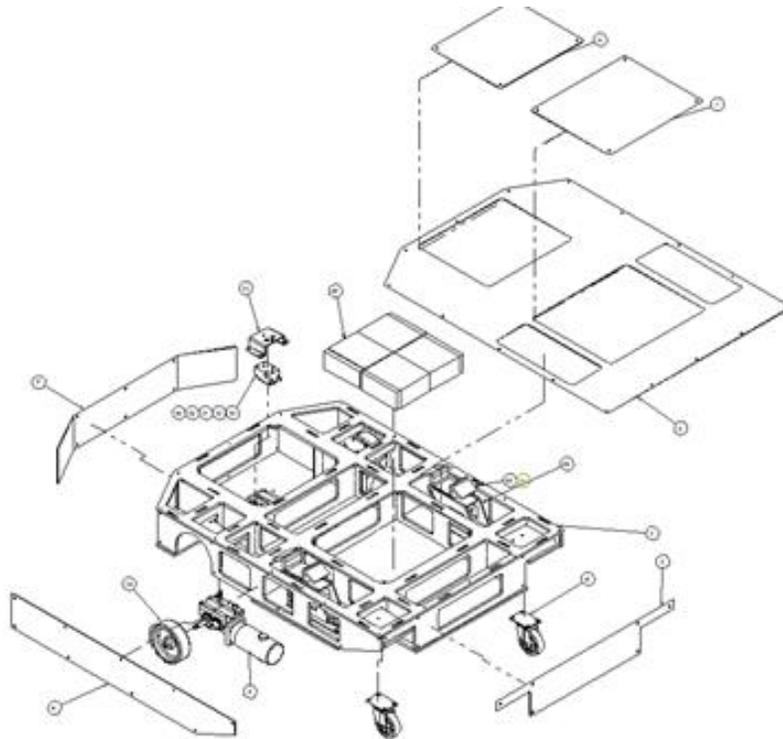
Figure 1: Assembly drawing of the Tugger Cart Assembly
