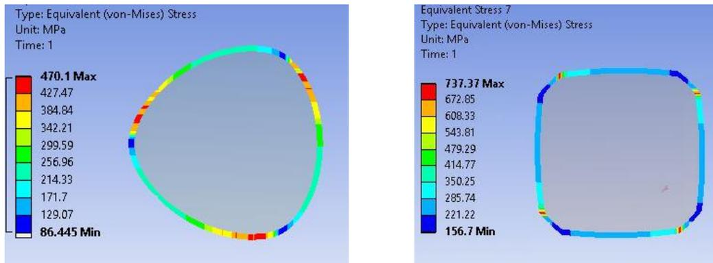
Figure 8: Distribution of von Mises stress along the edge
