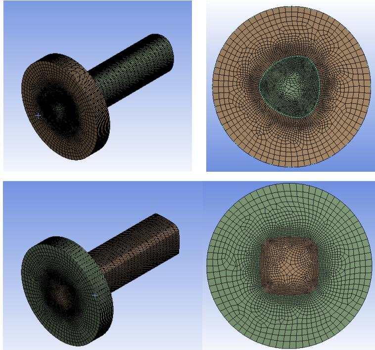
Figure 6: Meshing of three lobe and four lobe connections
