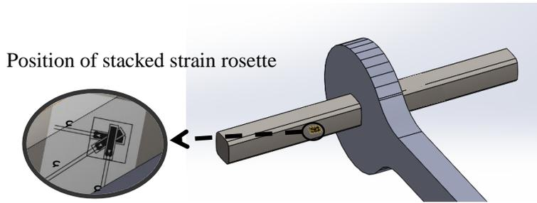
Figure 4: Position of strain gage in P4C shaft
