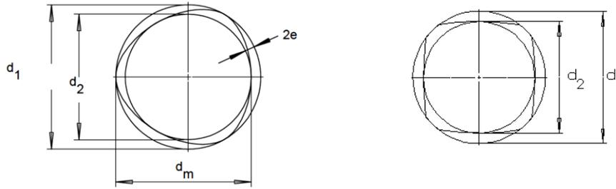
Figure 1: Profile parameters of the German DIN 32711 (P3G) and DIN 32712 (P4C) polygon standards.<sup>1,2</sup>
