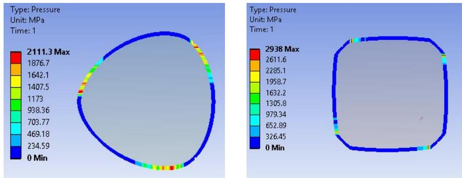
Figure 7: Contact stress distribution along the edge of the shaft hub connection
