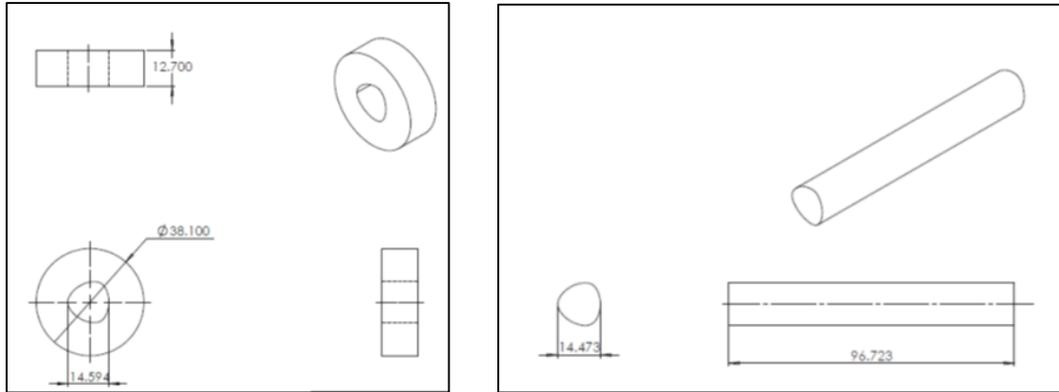
Figure 3: Dimension of P3G hub (left) and shaft (right)
