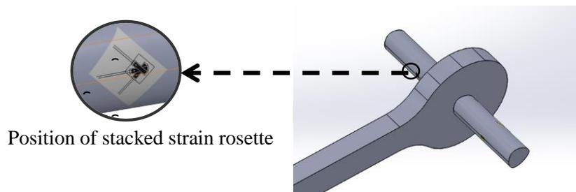
Figure 3: Position of strain gage in P3G shaft
