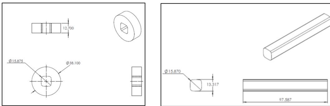
Figure 2: Dimension of P4C hub (left) and shaft (right)
