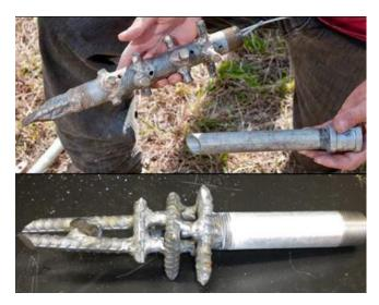
*Figure 3*. Drill bits utilized in this research (from top to bottom): Christmas tree, sand, and universal.
