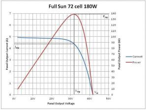
Figure 16 - Solar Panel Power Curve
