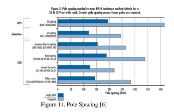
Pole spacing could be optimized if using a staggered distribution in a two way highway or roadway. A staggered distribution that the team will use for installation of the systems will be similar to the figure below.
