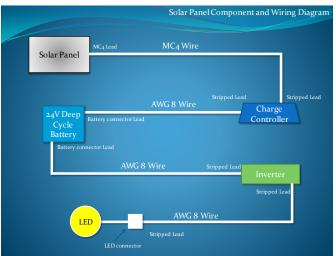
Figure 15: Solar Panel Component Wiring Diagram
