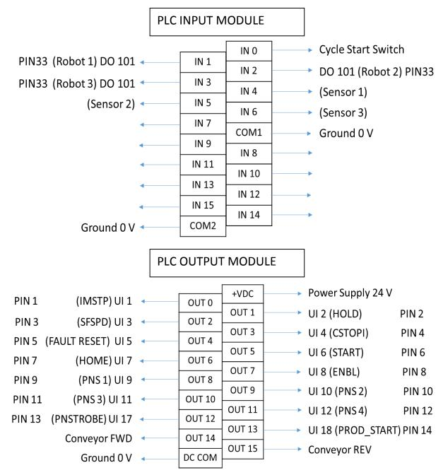
Figure 8. PLC I/O to UI/UO connections
