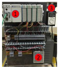
Figure 4. 1) Programmable Logic Controller, 1769-L32E 2) Switch Mode Power Supply, S82J-0224 3) Variable Frequency Drive, BMUD60-A2
