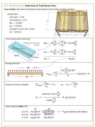
Figure 3 Beam Design with Tributary Area visualized
