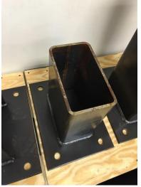
Figure 6: HSS Column and Baseplate Model
