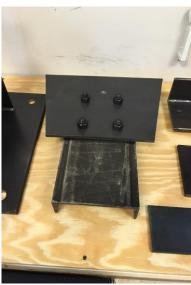
Figure 4: Bolted Channel-Plate Model
