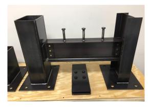
Figure 7: Composite Beam and Bolted Connection Model
