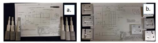
Figure 4: Lab 3 and 6, Fundamentals of Machining, a) lathe part, b) mill part. Students are required to machine both parts to spec.
