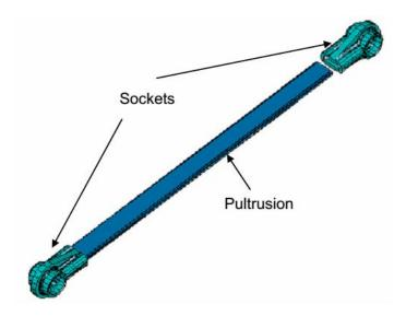
Figure 1 Connecting rod assembly
