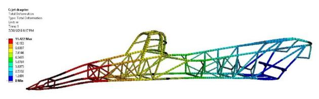
Figure 1: Static structural simulation of jet dragster impact
