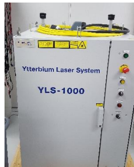
Fig. 3 High power (1 kW) laser for advanced laser applications.
