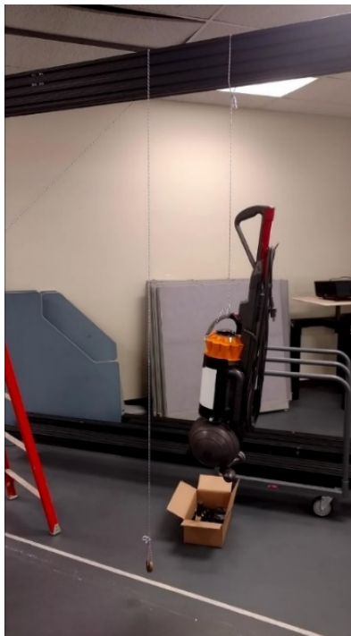
Fig. 3 Hanging vacuum to determine center of mass
