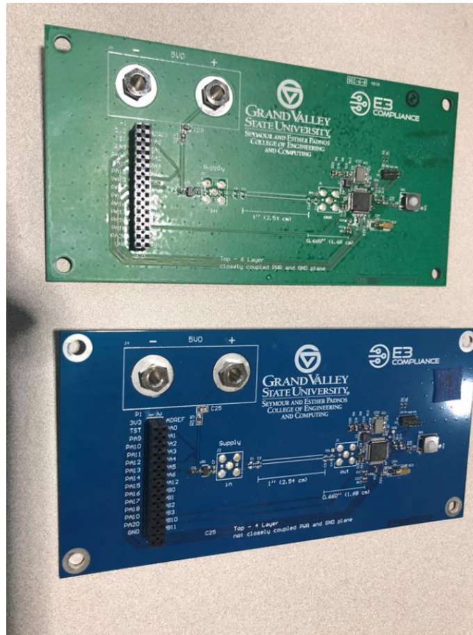
Figure 6: Four- and six-layer boards for decoupling capacitor study
