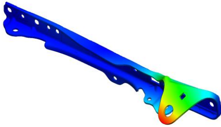
Figure 17. Mode 1: 465.16 Hz of Resonant Frequency
