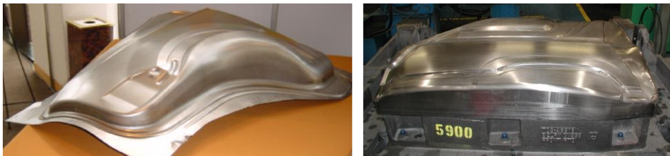
Figure 13. Example of an automotive fender and the die tool [14]
