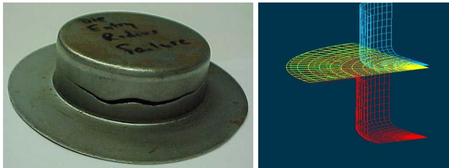
Figure 12. Failure of an example steel cup during drawing operation [14]
