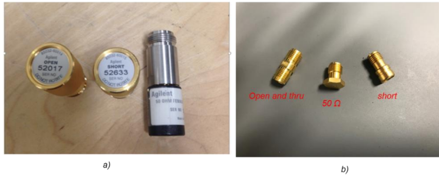
Figure 5: a) N-type calibration kit, b) SMA-type calibration kit
