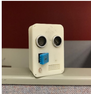
Figure 1: Lab in a Box with the ultrasonic sensor, temperature sensor, light sensor, microprocessor, and power supply.
