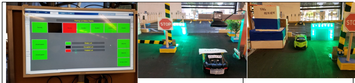
Figure 6: (a) User Display (b) Entry Gate opens for Valid Pass (c) Exit Gate Opens for no Violation
