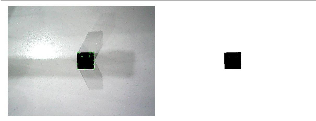
Figure 8. Object detection showing the corners detected (left) using the binary image generated (right)
