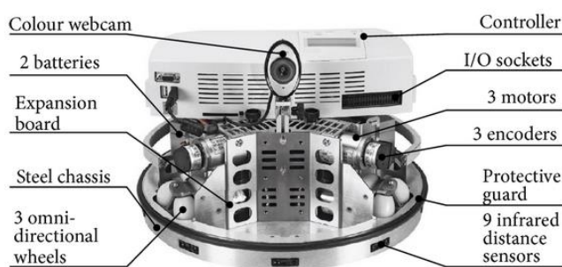
Fig. 2. Main components of the Festo Robotino mobile robot platform. Picture from Robotino Manual 24
